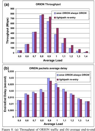
Figure 8: (a) Throughput of ORION traffic and (b) average end-to-enc delay, versus average load for the two policies.
